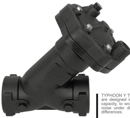
TYPHOON Y Type Plastic Automatic Hydraulic Control Valves are designed in "Y" body model type, with high modulation capacity, to work with minimum pressure loss, cavitation and noise under difficult working conditions with high pressure differences.
