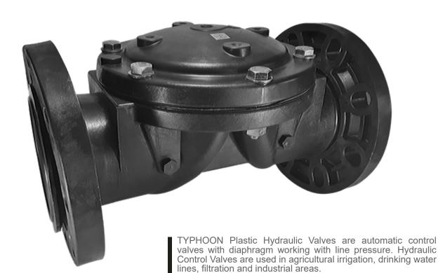
TYPHOON Plastic Valves are automatic control valves with diaphragm closure working with line pressure. Valve body and diaphragm design ensure smooth flow with minimum pressure loss. Since there is no bearing, bush and shaft in the valve body, valve life is longer. The only moving part of the valve is the diaphragm.
