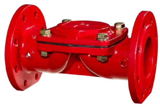
Typhoon hydraulic control valves are automatic valves with direct diaphragm shut-off working with line pressure. It is a comfortable, smooth flow in the minimum pressure loss of the body and diaphragm, which is kept in the foreground in its design.
